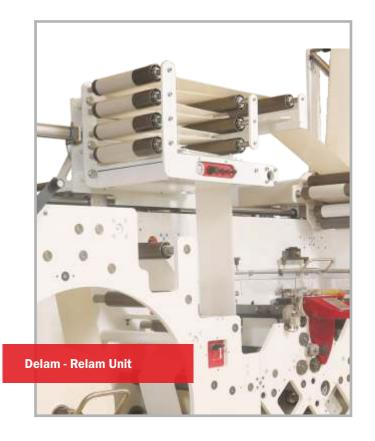
Delam - Relam unit on rails separates the liner from the self-adhesive material to allow printing on the adhesive. The adhesive printed section is dried before being relaminated.
