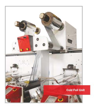
Cold foil stamping on rails allows stamping of glossy metallic effects with lower plate costs and higher speeds, using a flexo station.
