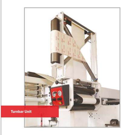
Turnbar unit on rails allows for flipping the web and allows for printing on the reverse side of the web.
